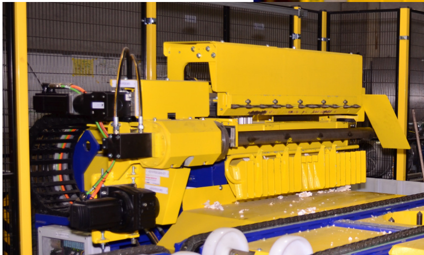
Coiling shaft with clamping device
